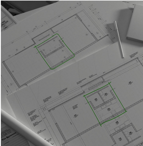
Figure 6. The Utility Core as Shown in the Build Set (Top Left) and Permit Set (Bottom Right). / Rendering by author.
