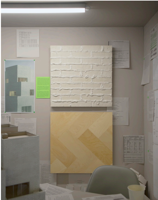
Figure 7. Weeping Joint and Parquet Floor Material Mockups. / Photo- graph by author.
